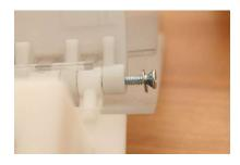
Add the screw between both links using a screwdriver and have a washer and bolt ready to the other side
